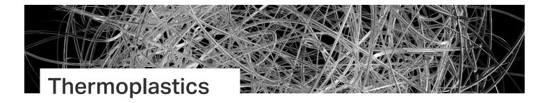
Thermoplastics are one of the most common material groups in additive manufacturing. Thermoplastic 3D printing processes involve heating a plastic material to just below its melting temperature where it is semi-formable to create a shape. Thermoplastics are tough but weak, deforming rather than fracturing under stress. They have relatively low melting points, and low chemical and abrasion resistance.
